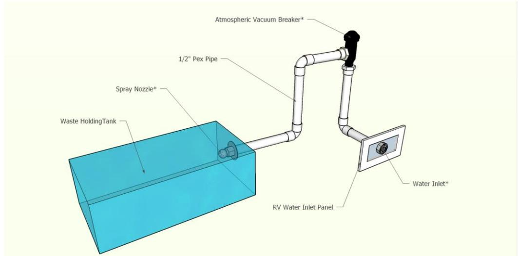
Notes: QAI's certification does not cover the final assembly of the Wasteholding Tank Flushing System. All components used in the final assembly of the system must be installed in accordance with all requirements of IAPMO TS 27, CSA Z240RV Series, and NFPA 1192.
