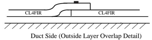
**Product: CL4FIRE 6 pcf. density, 2-layers of of 38mm (1 1/2'') for an overall thickness of 76mm (3'')**
