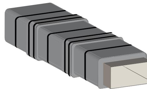
**Single Layer System with 6 inch (152 mm) Collar and 3 inch (76 mm) Overlap Installation**
