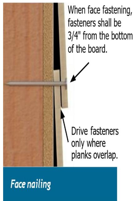
Figure 2. Allura® Lap Siding Face Nail Fastening Details
