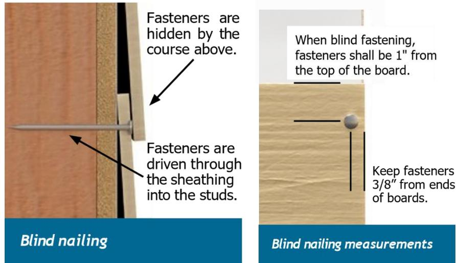
Figure 1. Allura® Lap Siding Blind Nail Fastening Details
