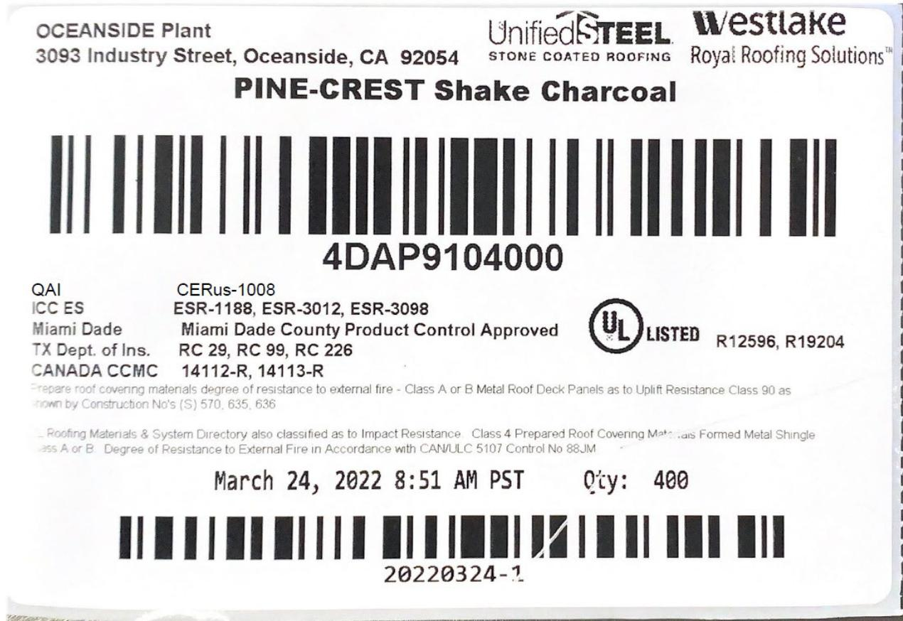
Figure 1. Representative Example of Unified Steel™ Stone Coated Metal Panels Labels
