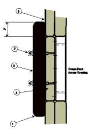
For installation over a standard NFPA-96 installed grease duct access door assembly or alternately can be installed over a ventilation air duct access door assembly.
