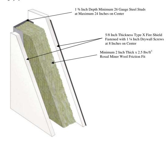
The joint details of Panel Built 1 Hour Fire Rated Walls are Shown Below.
