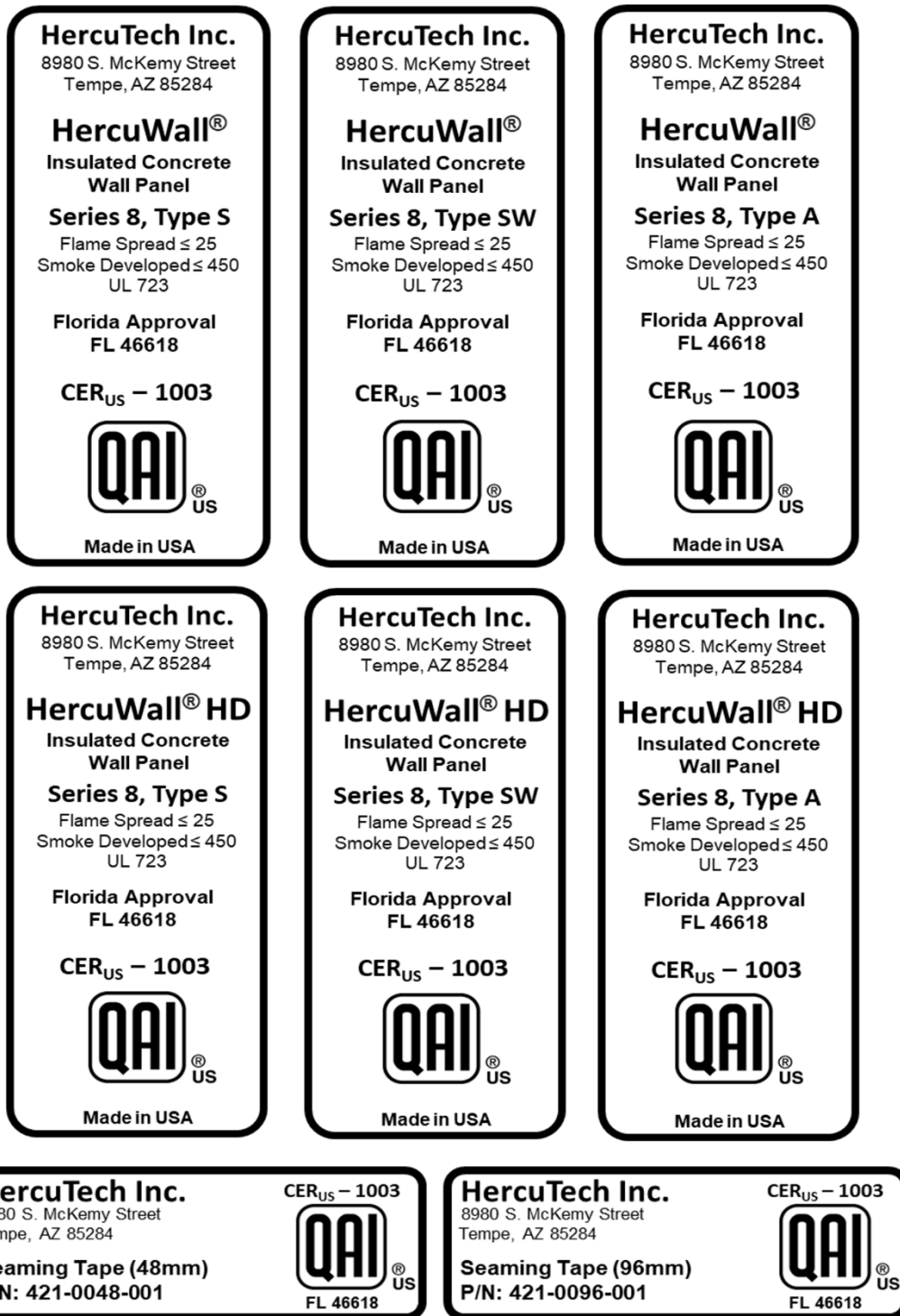
Figure 1. Example of HerculWall®, HerculWall® HD Series 8 Panels, Posts and Seam Tape Labels
