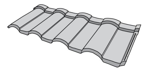
Figure 4 – BARREL VAULT TILE
