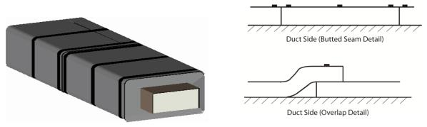
Product: CL4FIRE 6 pcf. density, 1-layer of of 76mm (3") for an overall thickness of 76mm (3") thick
