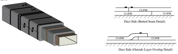
Product: CL4FIRE 6 pcf. density, 2-layers of of 38mm (1 1/2") for an overall thickness of 76mm (3") thick
