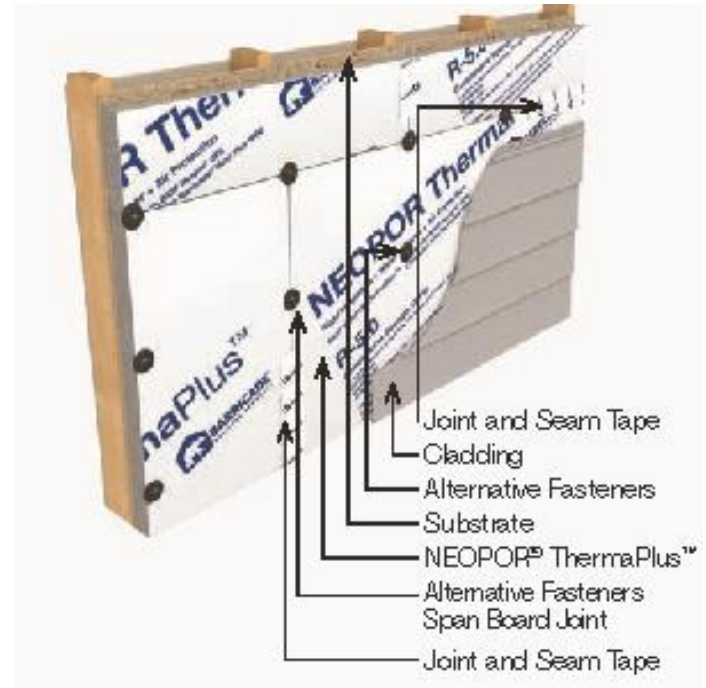
Figure 2. Alternate NEOPOR ThermaPlus™ Installation with Fastener Washer Spanning Joint.
