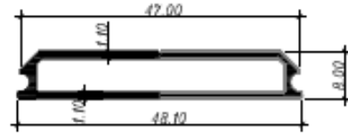
CODE : C-018 PROFILE : Back Cover 2" WEIGHT : 0.344kg/m
