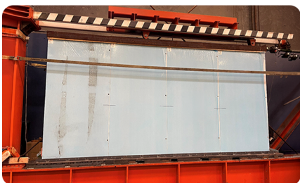
Racking shear testing establishes wall panel design values
